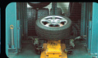
10 Impact Tester Simulating side impact with weight up to 830 kg (passenger cars VIAUM)
