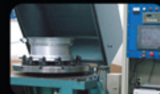
Cornering Bending Endurance Tester Simulating cornering loading conditions by subjecting to yaw and rotating bending loads at 750 kph
